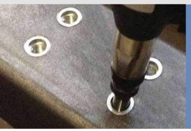
Special accessories, nosepieces and mandrels, for example, extended, or for UNC/UNF coarse threads or for inside riveting locations are available on request.
